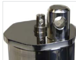
Liquid flows in when the sampler hits the bottom
