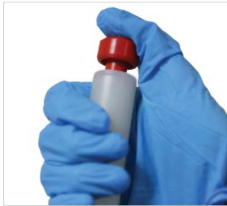
Push Button to open the valve in the tip and take the sample
